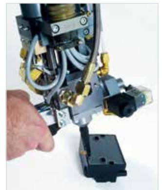
Manual application of potting compound with the SONDERHOFF MK 50
