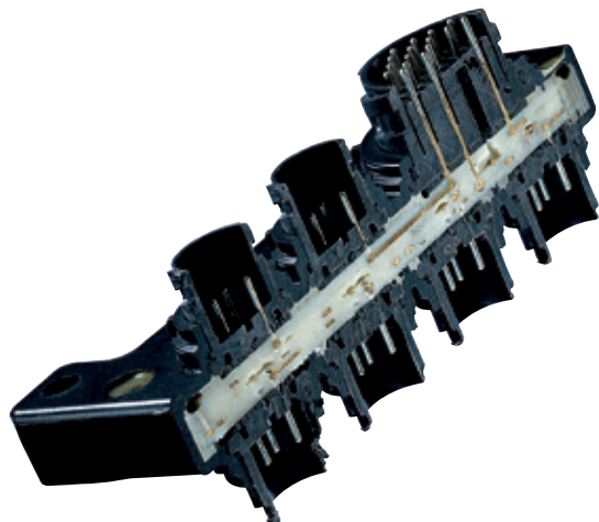
Potting of an automotive connector plug
