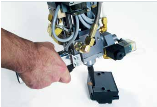
Manual potting of an electronic component with SONDERHOFF MK 50 and the 2-component casting resin SONDERHOFF FERMADUR
