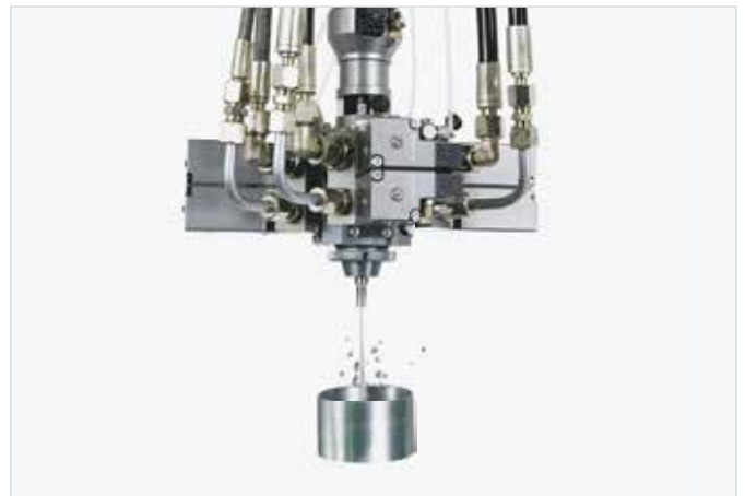
SONDERHOFF MK 400 with high-pressure water rinsing
