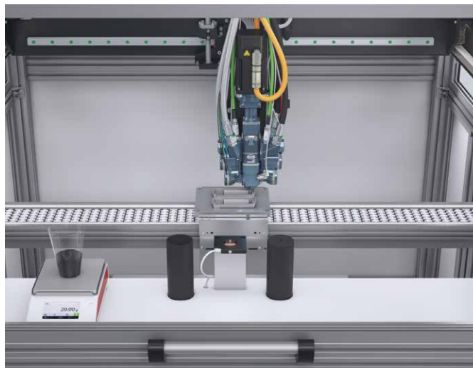
Workpiece carrier stops at the centering device
