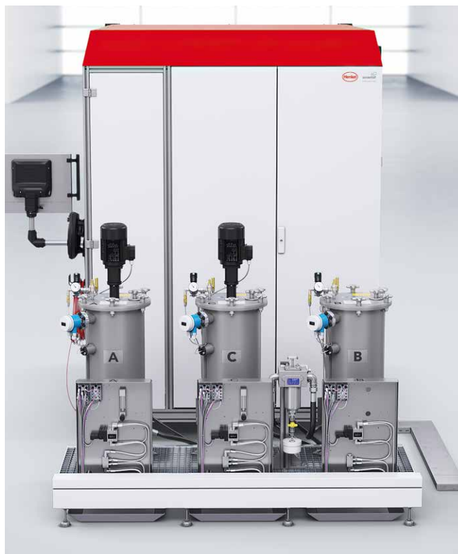
Dosing machine cabinet integrated in the rear of the cell with hinged doors and material pressure tank (24 l or 44 l, single-walled or double-walled) on grating platform with adjustable leveling feet and drip tray
