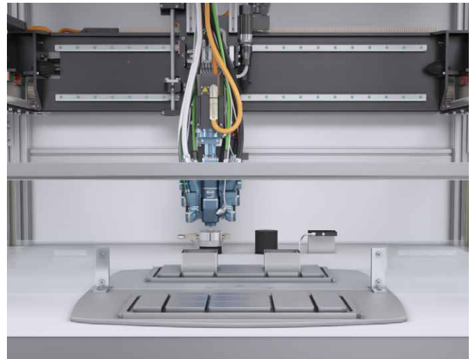
Mixing head during filling shot in the AIR-CLEAN device
