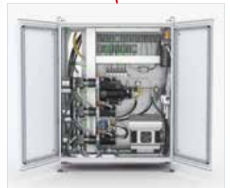
The dosing machine cabinet contains the components of the dosing periphery, e.g. the dosing pumps.
