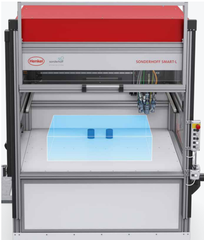
Travel range in the SONDERHOFF SMART-L dosing cell: 1,000 x 800 x 250 mm (x/y/z)
