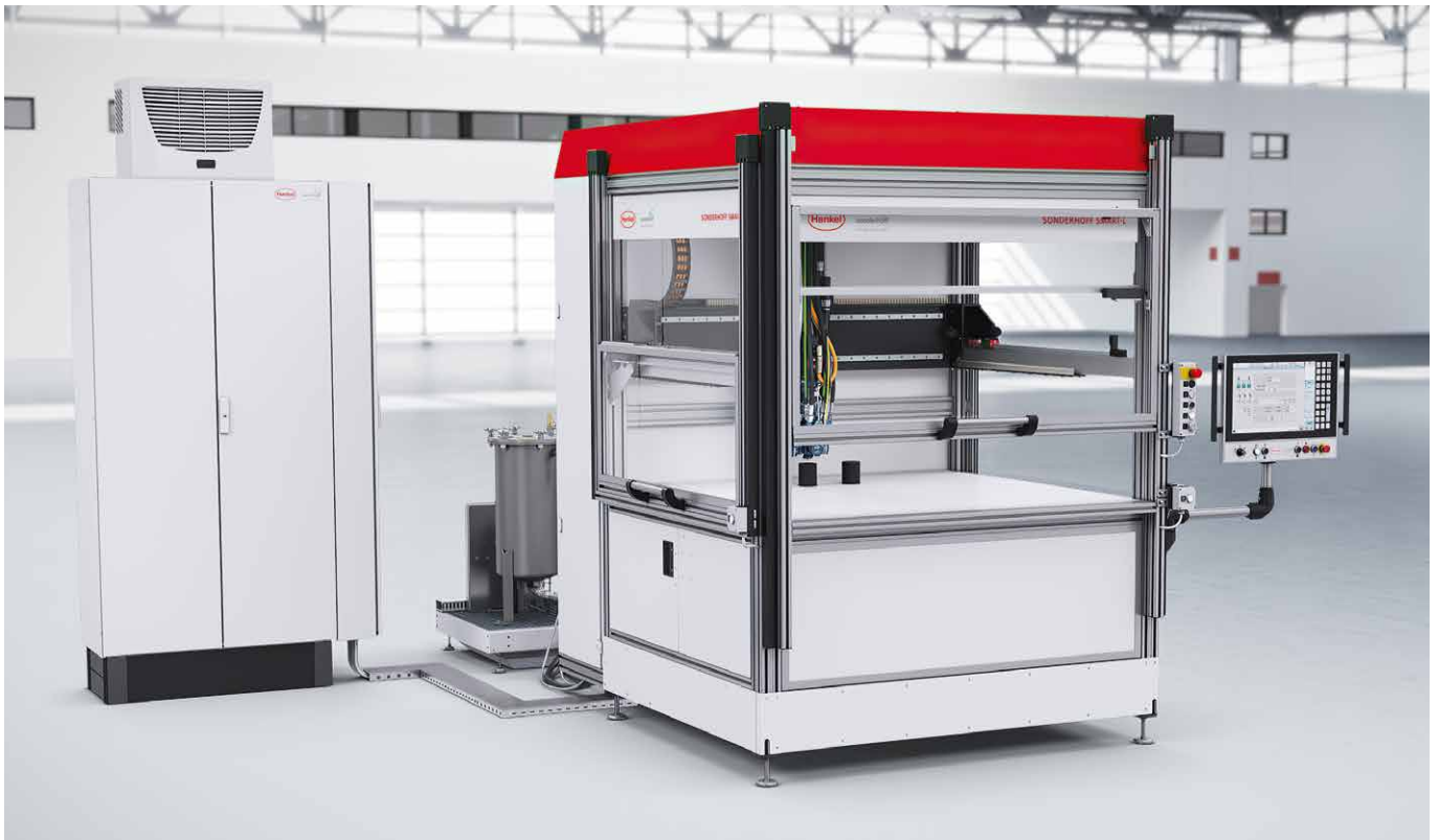
SONDERHOFF SMART-L dosing cell with lifting door and MK 825 PRO mixing head, configured for two or optionally three material components, as well as material pressure tank at the rear of the cell and switch cabinet for the control system
