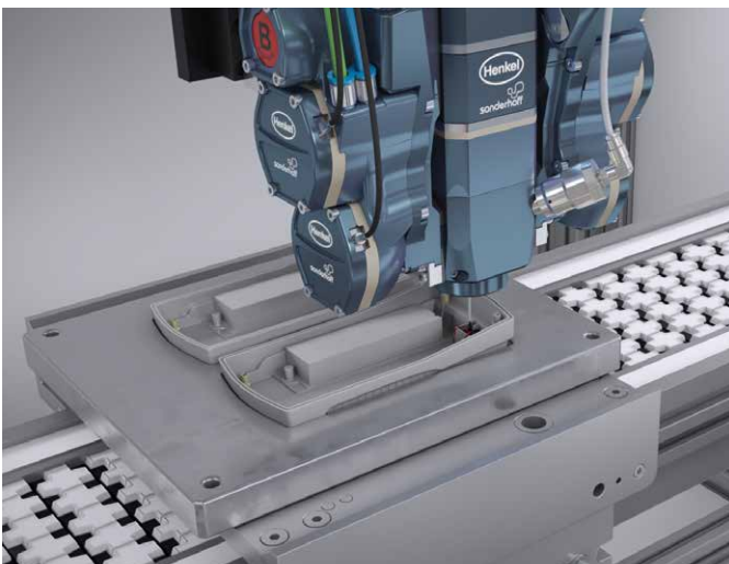
The CNC-guided mixing head precisely positions itself above the component and doses the potting compound.
