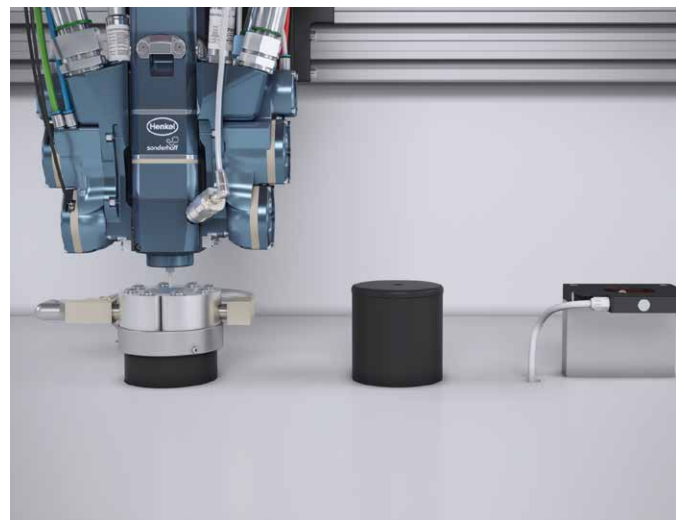
Left Side: The pneumatic AIR-CLEAN nozzle cleaning system cleans the mixing head nozzle by means of compressed air. Middle: Device for high-pressure water rinsing and filling shot station. Right Side: The NOZZLE-CONTROL laser-based nozzle measuring unit checks that the dosing nozzle is in the correct position and there is no contamination.
