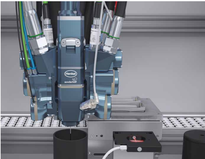
The MK 800 PRO mixing head is in the filling shot position.
