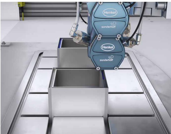
Dosed application of FERMAPOR K31 foam sealant into the groove of the filter frame
