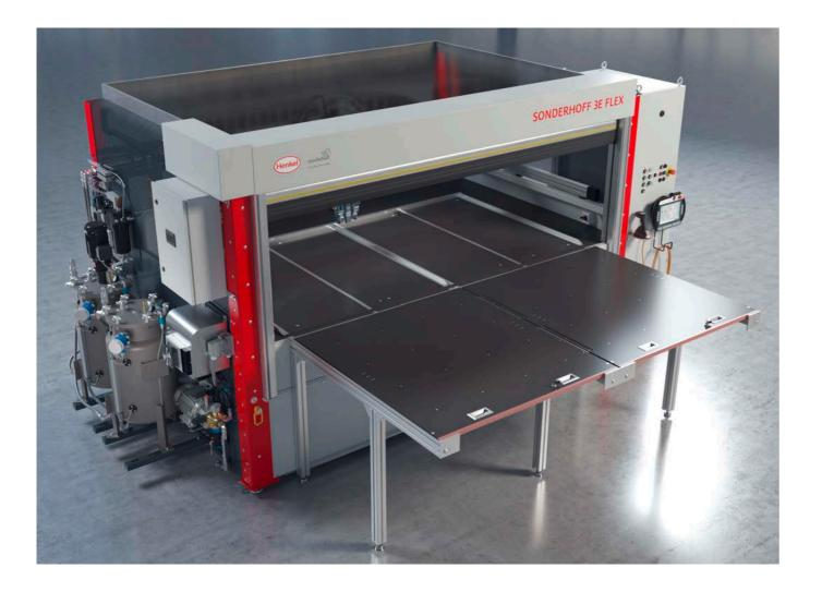
The parts can also optionally be loaded via an attachable sliding/shuttle table by manually moving the mounting plates.
