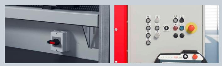
Switch for "mixing head maintenance position" preselection
