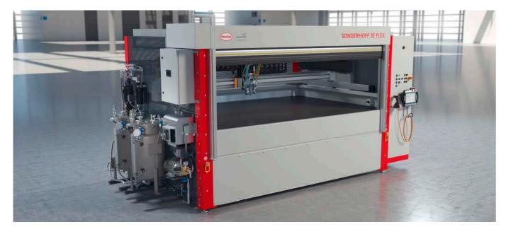
The MK 800/825 PLUS precision mixing head is used in the SONDERHOFF 3E FLEX dosing cell for processing a 2K material system. In the mixing head, the material components are mixed dynamically and homogenously and then precisely dosed for application on the component. The MK 800 PLUS has a dosing capacity of 3.0 to 100 g/s and the MK 825 PLUS from 0.2 to 3.0 g/s, with an infinitely adjustable mixing ratio of 10 : 1 to 1 : 2 and a dosing accuracy of  $\pm$ 1%.
