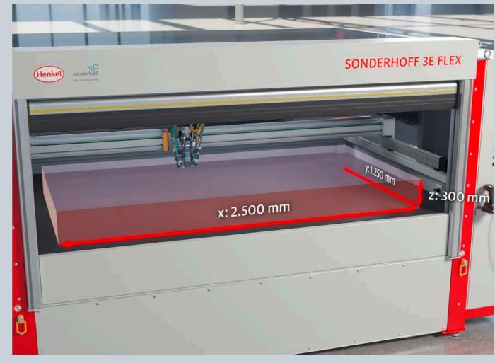
To produce oversized parts with a maximum dimension of 2,500 x 1,250 x 300 mm (3E FLEX) the two sliding table plates are joined for one large mounting plate.
