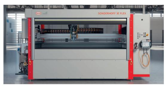
Front of the 3E FLEX with upper, removable cover plate. Tabletop height 1,000 mm.
