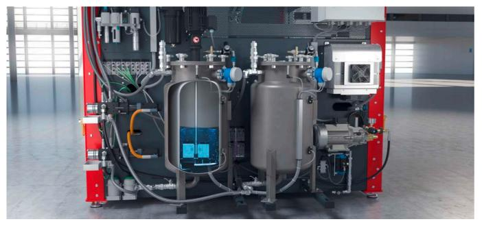
The air loading in the material pressure tank helps to create the desired physical properties and cell structure of the foam. The density can be influenced by adding compressed air to the material component.
