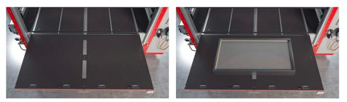
The two mounting plates are connected by couplers so that one large sliding table can be formed.
