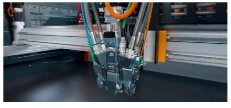
Standard equipment: Precision mixing head MK 800/825 PLUS for 2 components, with high-pressure water rinsing.
