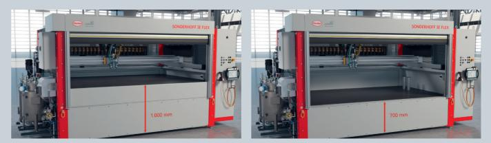
The standard height of the work table is 1,000 mm. With the 3E FLEX, it can be adjusted down to 700 mm.
