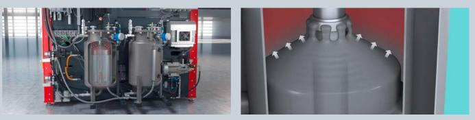
Material is continuously conveyed from the bottom of the pressure tank through a riser pipe and fed back onto the conical surface as a thin film. This process continuously reduces and completely dissolves air bubbles in the material.
