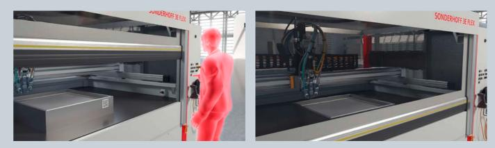
To remove one or more parts after dispensing, the high-speed door opens automatically The high-speed door in closed state. or the operator opens it by pressing a button
