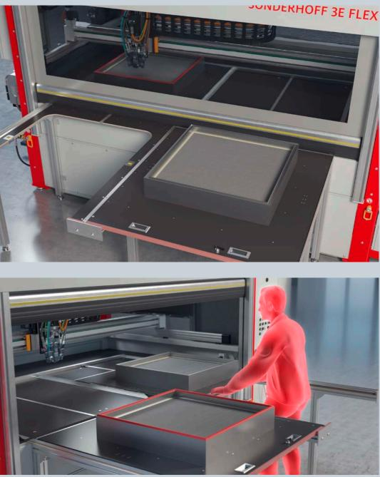
After the dosed application, the machine operator opens the high-speed door and pulls the sliding table with the finished parts out of the working area for removal.
