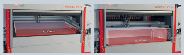
The standard component height to be processed with the 3E FLEX can be extended from 300 mm to 600 mm.
