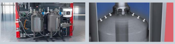
Material is continuously conveyed from the bottom of the pressure tank through a riser pipe and fed back onto the conical surface as a thin film. Due to the air loading, the density changes and the material becomes lighter in color.
