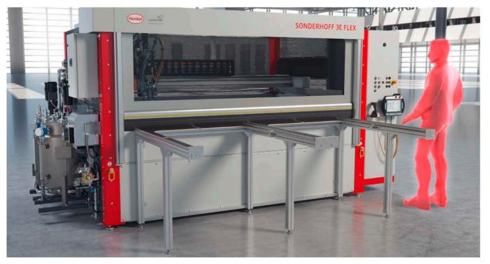
With all three 3E dosing cell variations, the two mounting plates can be connected to form a single large sliding table for material application on oversized parts.
