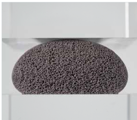
Cross-section of a polyurethane foam bead – uncompressed
