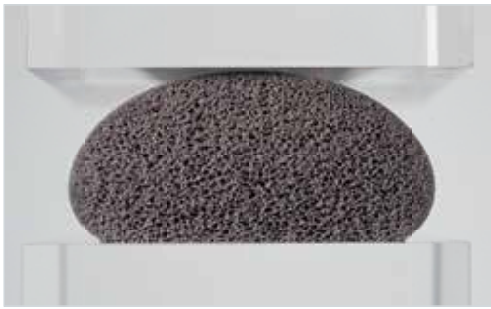
The unpressed polyurethane foam gasket before installation.
