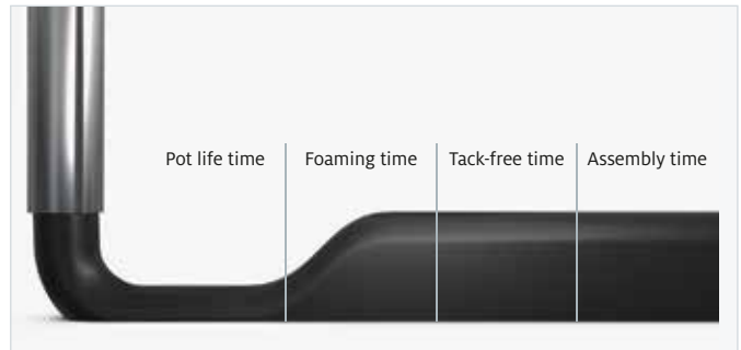
The different reaction phases of the sealing foam in the chronological sequence
