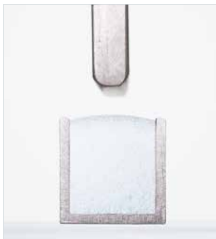
Cross-section of a silicone foam bead in the groove without pressing
