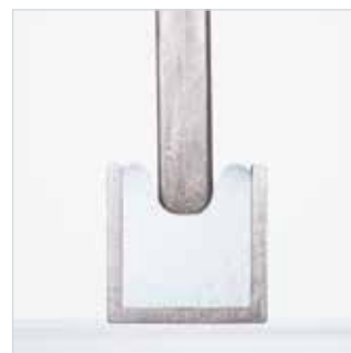
Cross-section of a silicone foam bead in the groove and pressed to approx. 30 %
