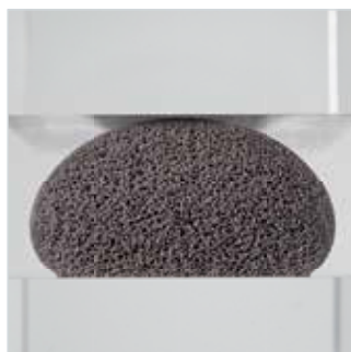
Cross-section of a polyurethane foam bead – uncompressed
