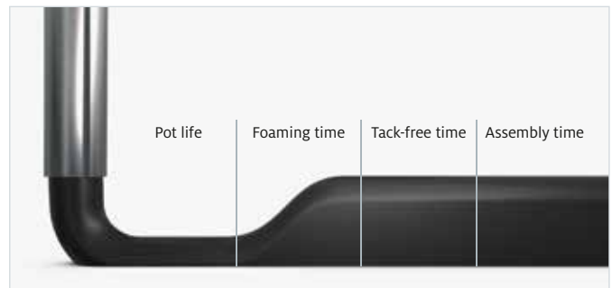
The different reaction phases of the sealing foam in the chronological sequence
