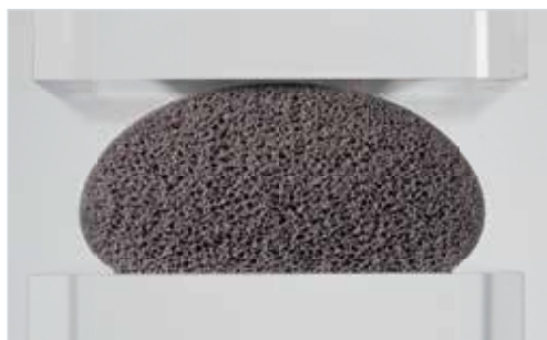
The unpressed polyurethane foam gasket before installation.
