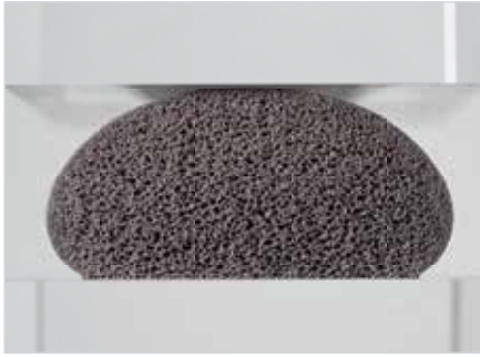
Cross-section of a polyurethane foam bead – uncompressed
