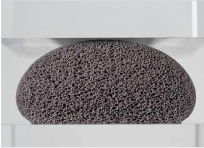
Cross-section of a polyurethane foam bead – uncompressed
