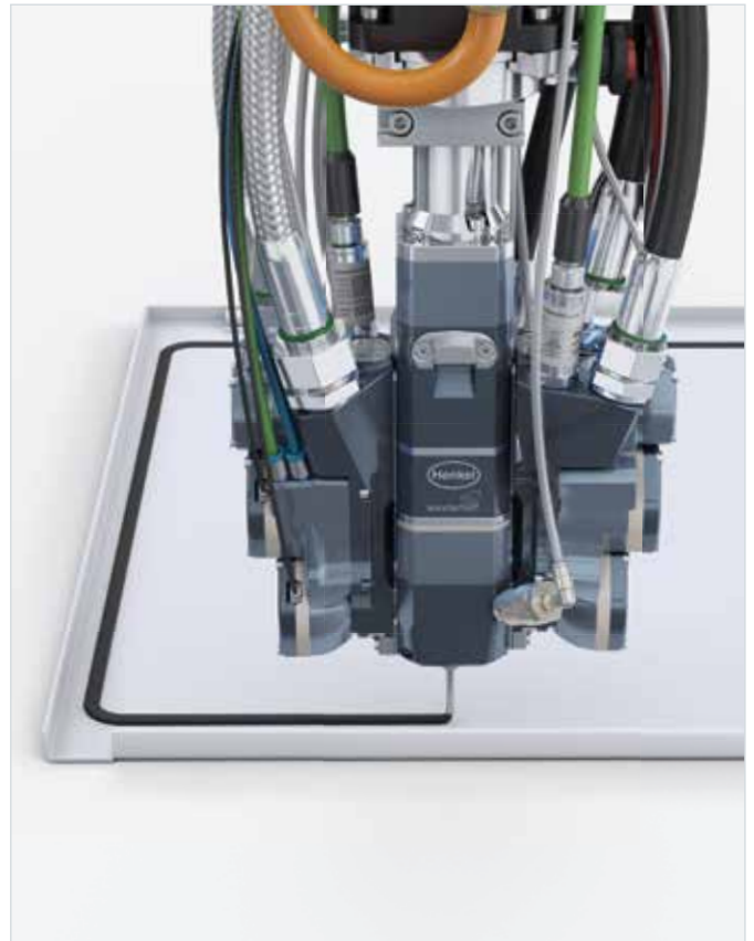
Application of PU foam gasket to an HVAC panel
