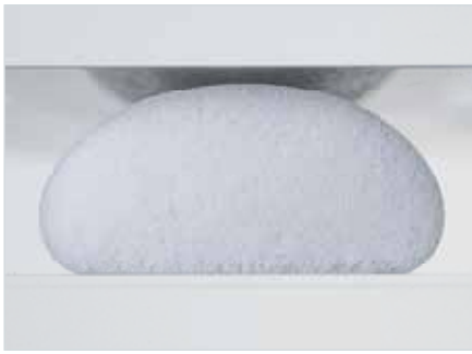
Cross-section of a silicone foam bead – uncompressed
