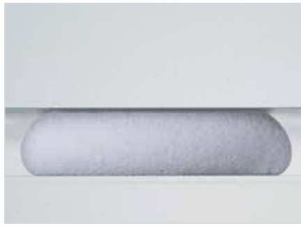
Cross-section of a silicone foam bead with 30% compression
