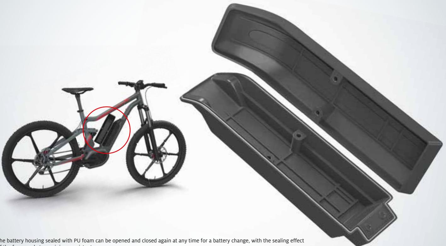
The battery housing sealed with PU foam can be opened and closed again at any time for a battery change, with the sealing effect of the foam gasket remaining consistent.
