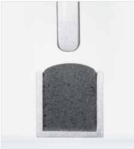
Cross-section of a polyurethane foam bead in the groove without compression
