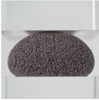
Cross-section of a polyurethane foam bead – uncompressed
