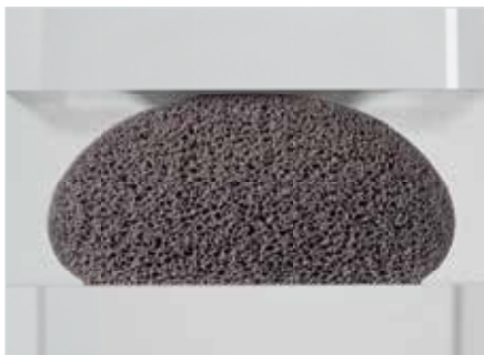
Cross-section of a polyurethane foam bead – uncompressed
