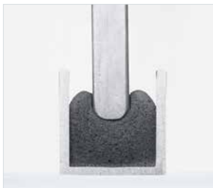
Cross-section of a polyurethane foam bead in the groove and compressed to approx. 50%
