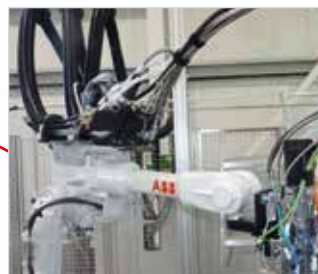
The 6-axis robot guides the mixing head precisely over the contours of the component during the dosing process.
