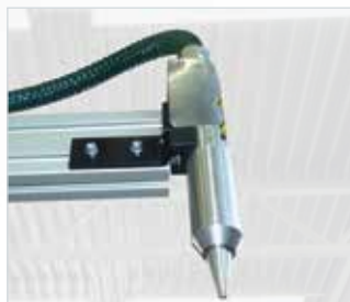
The optional plasma nozzle mounted on the robot arm applies the plasma parallel to the seal application on plastic surfaces of the component in the same contour.
