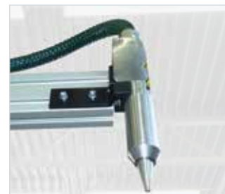
The optional plasma nozzle mounted on the CNC linear robot applies the plasma before the seal is applied.
