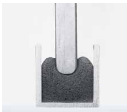
Cross-section of a polyurethane foam bead in the groove and pressed to approx. 50 %
