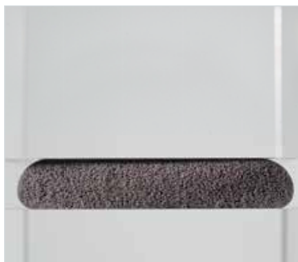
Cross-section of a polyurethane foam bead with 50% compression
