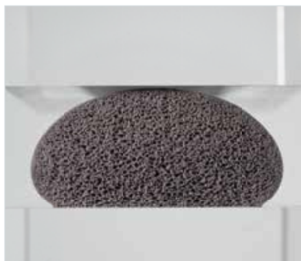
Cross-section of a polyurethane foam bead – unpressed
