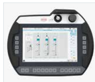
The multifunctional Mobile Panel MP 2 (10.1" WXGA TFT) enables convenient operation of the dosing system.
