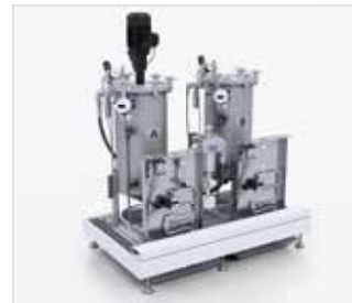
Separate standing material pressure tanks (24 L or 44 L, single-walled or double-walled) with capacitive minimum fill level sensors, on grating platform, with adjustable leveling feet and drip pan
