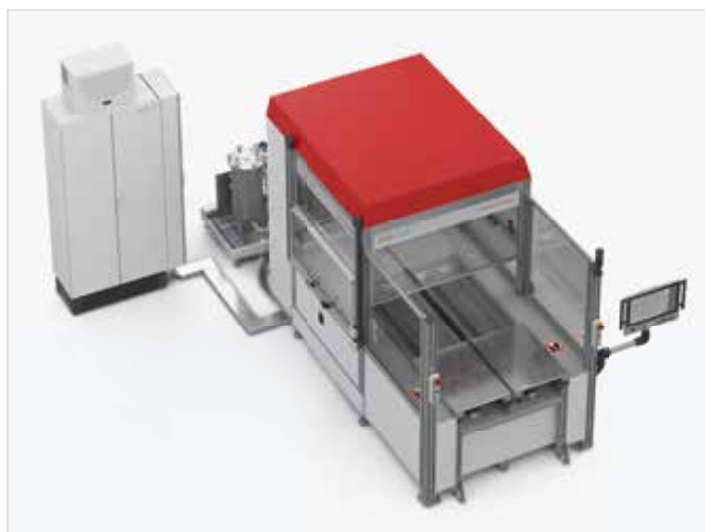
Alternative reference system of the SMART-L dosing cell with sliding table . Two shuttle tables operating in pendulum mode enable the parts to be processed on one level. This means that very short cycle times and continuous operation can be guaranteed.
