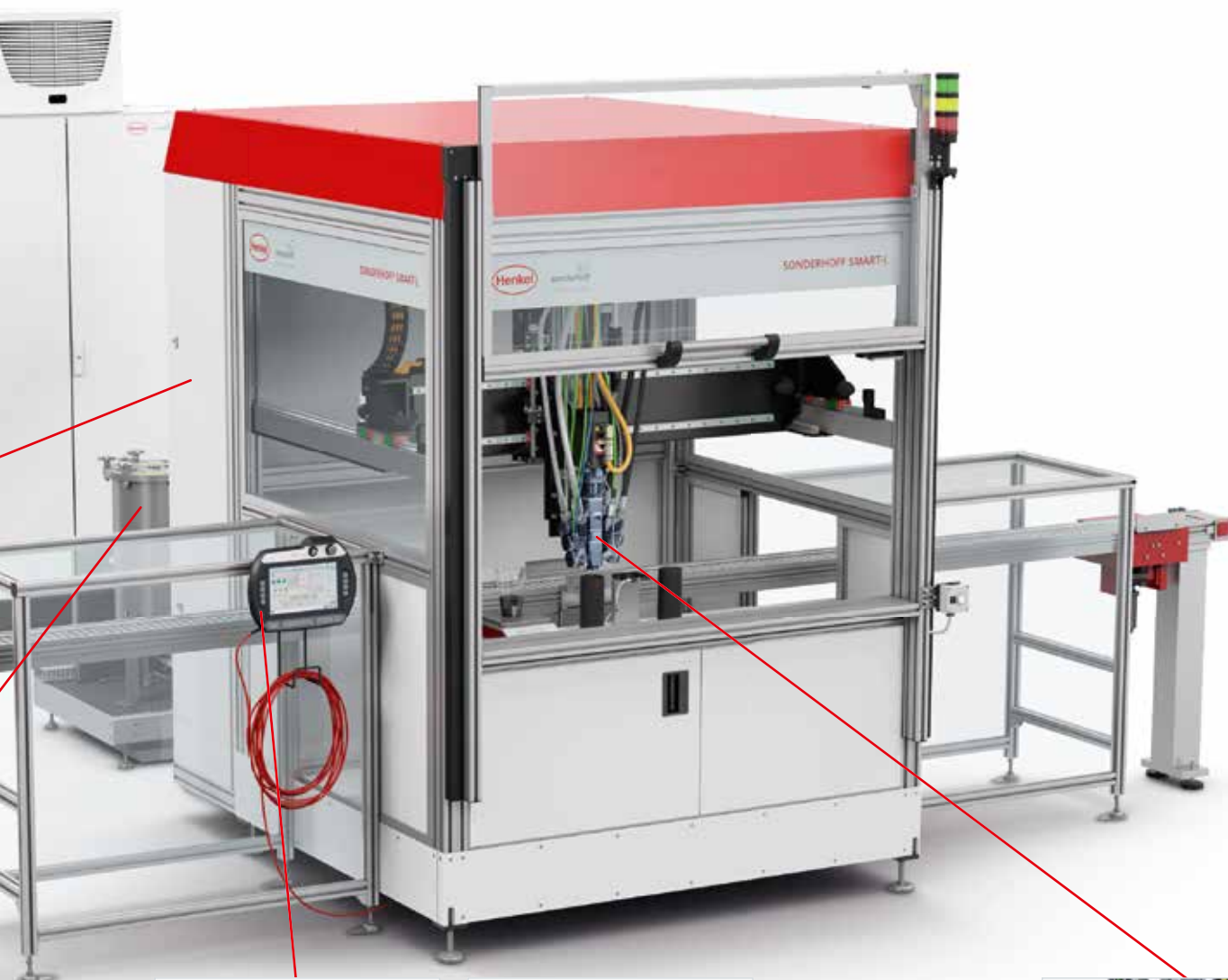
Alternative reference system of the SMART-L dosing cell with sliding table . Two shuttle tables operating in pendulum mode enable the parts to be processed on one level. This means that very short cycle times and continuous operation can be guaranteed.
