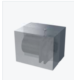
Two-part mold for the production of a cable grommet
