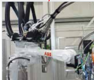
The 6-axis robot guides the mixing head precisely over the contour of the cable grommet during the dosing process.
