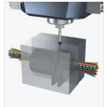
The mixing head doses PU potting material into the molding tool
