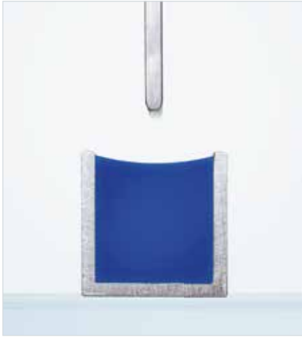
Cross-section: Polyurethane gel in groove
