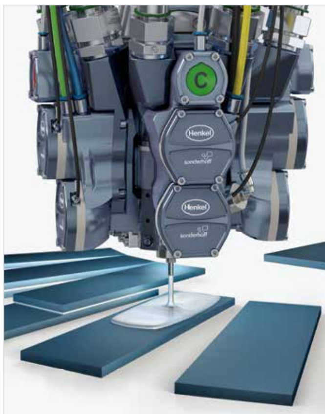
Full-surface bonding with FERMADUR adhesive sealants
