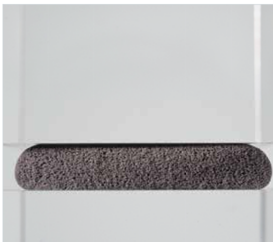
Cross-section of a polyurethane foam bead with 50% compression
