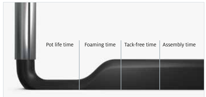
The process sequence for forming a foam gasket
