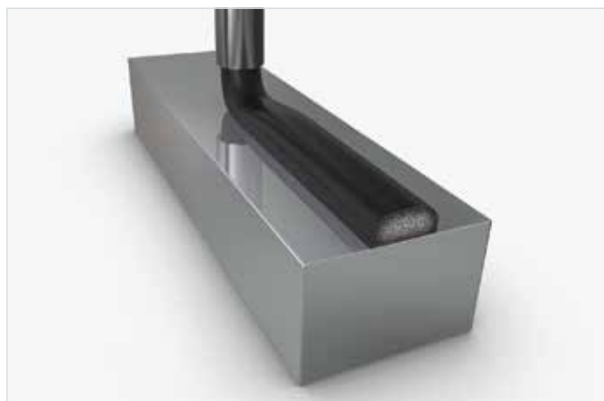
The process sequence for forming a foam gasket
