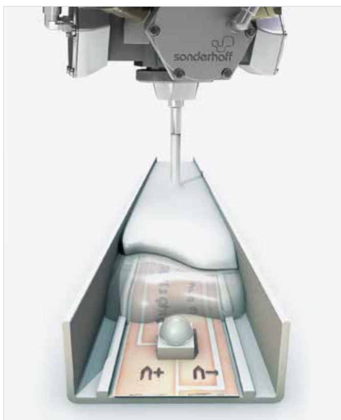
Potting of LED light fixtures with transparent and translucent FERMADUR
