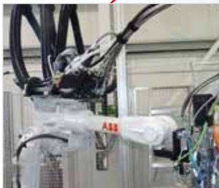
The 6-axis robot guides the mixing head with repeated accuracy over the charging plug housing for precise potting of the cable strands with the connector.
