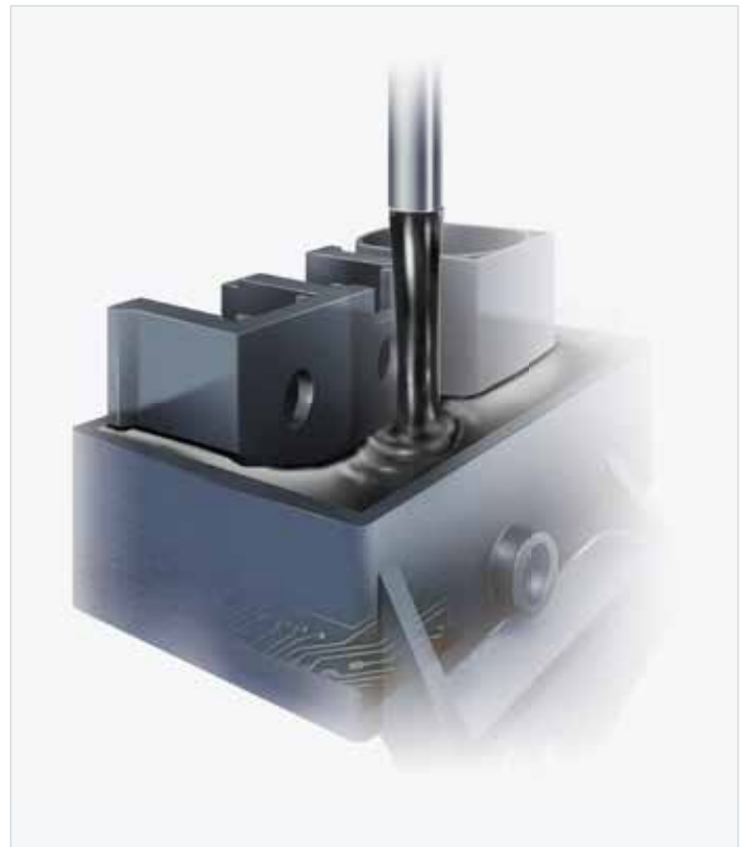
Dosing of polyurethane potting compound into the component via the CNC-controlled mixing head of the DM 502 dosing system
