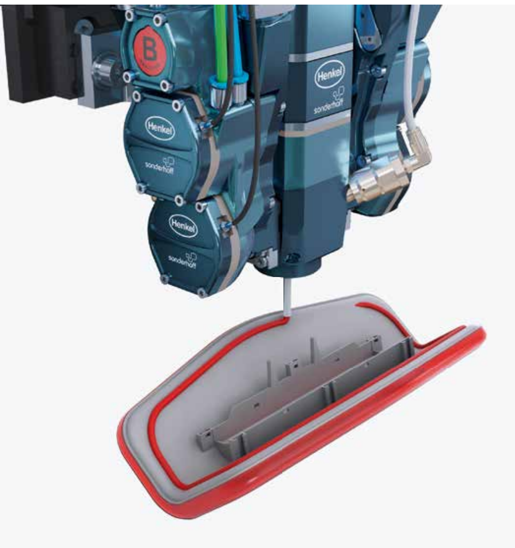
3D third brake light, without groove, with red polyurethane foam gasket
