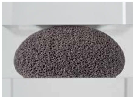
Cross-section of a polyurethane foam bead – uncompressed
