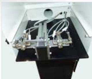
The optional primer nozzle mounted on the robot arm applies the primer parallel to the seal application on powder-coated or stainless steel surfaces in the same contour.
