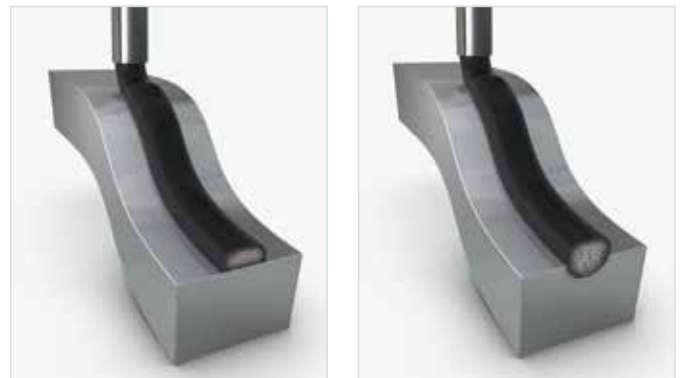
The different reaction phases of the sealing foam in the chronological sequence
