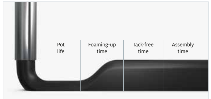
The different reaction phases of the sealing foam in the time sequence.
