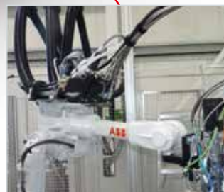
The 6-axis robot guides the mixing head for dosing application precisely over the housing contour.
