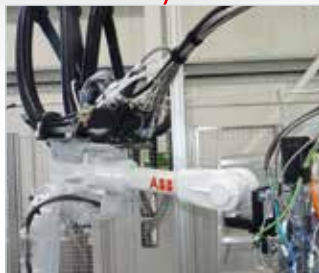
The 6-axis robot guides the mixing head precisely over the housing contours during dosing application.
