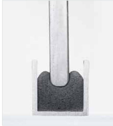
Cross-section of a polyurethane foam bead in the groove and compressed to approx. 50 %
