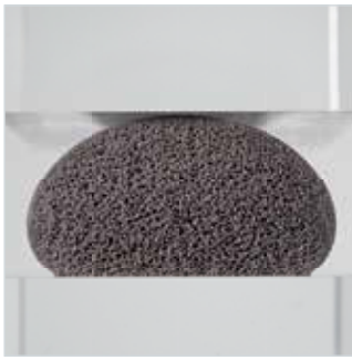
Cross-section of a polyurethane foam bead – uncompressed
