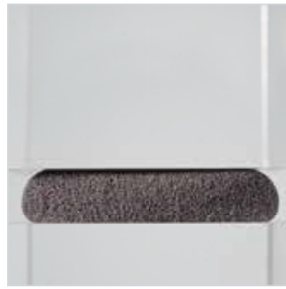
Cross-section of a polyurethane foam bead with 50% compression
