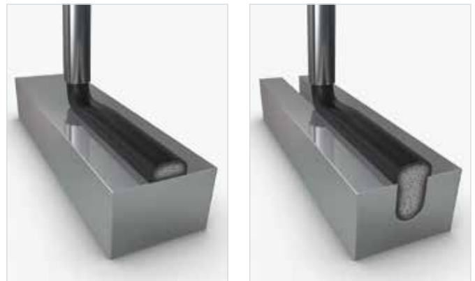
The different reaction phases of the sealing foam in the chronological sequence
