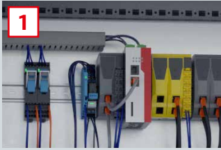
VPN router for remote maintenance (remote collaboration)
