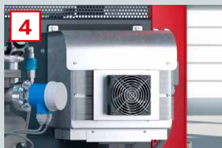
Peltier unit for cooling the MK 825 PLUS precision mixing head
