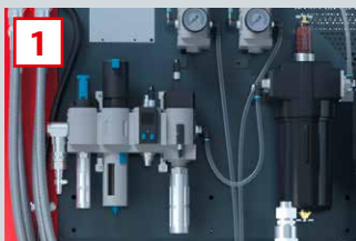
Compressed air connection, dryer and maintenance unit
