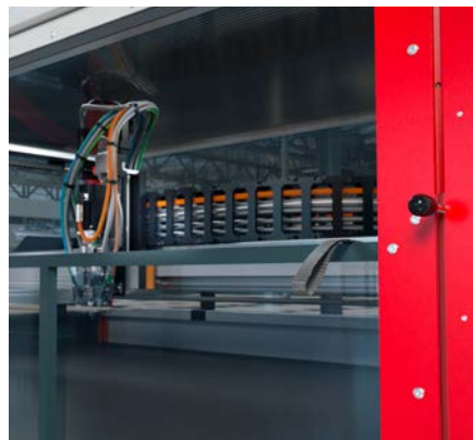
Half-open lifting door showing the MK 825 PLUS precision mixing head and the energy chain
