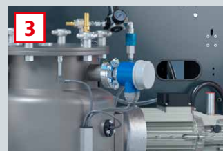
Overfilling protection for the use of an optional refilling station
