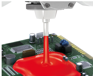
E-Mobility batteries Potting
