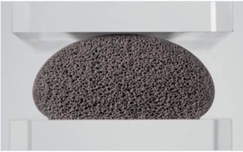
The unpressed polyurethane foam gasket before installation.
