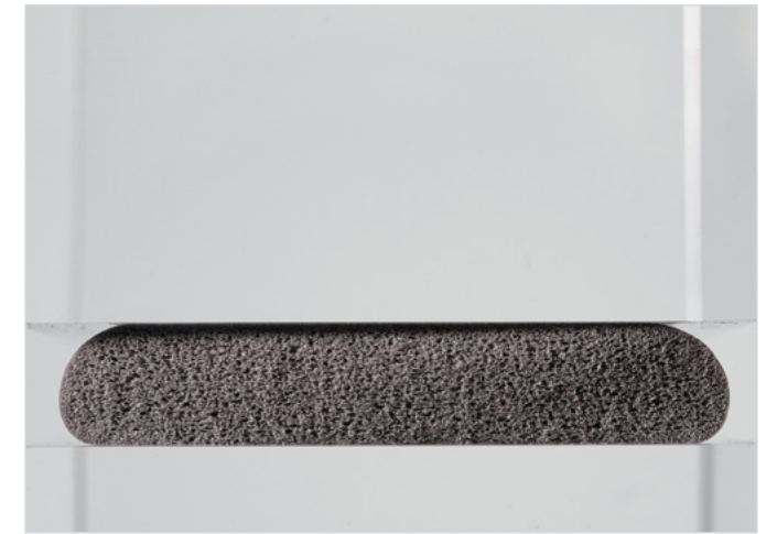
Cross-section of a polyurethane foam bead with 50% compression
