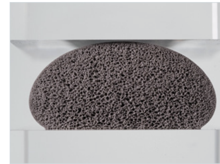
Cross-section of a polyurethane foam bead – unpressed
