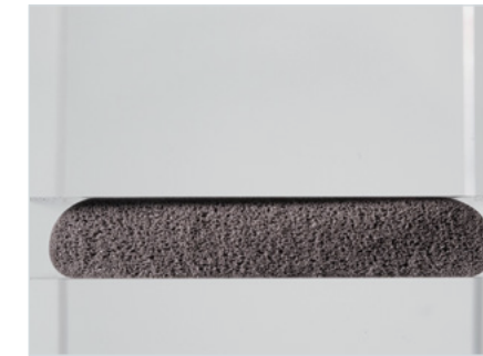
Cross-section of a polyurethane foam bead with 50% compression
