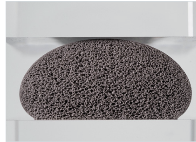
Cross-section of a polyurethane foam bead – unpressed
