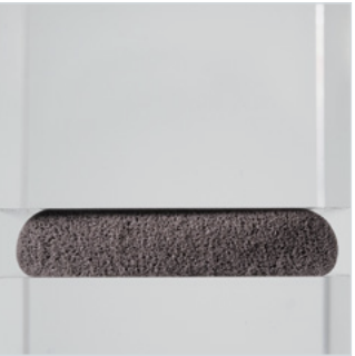
Cross-section of a polyurethane foam bead, compressed to 50%
