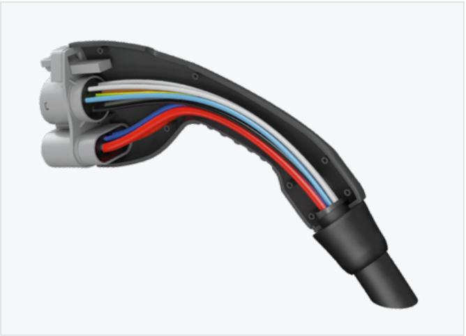
Cross-section of EV charger connector with waterproof potted cable strands
