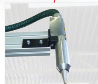
The plasma nozzle , optionally mounted on the CNC linear robot, applies the plasma before the seal is applied.
