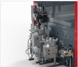
The material pressure tanks , with 44 l capacity for the A component and 24 l for the B component, accommodate the typical, asymmetrical mixing ratio, which can be continuously adjusted from 10 : 1 to 1 : 2.
