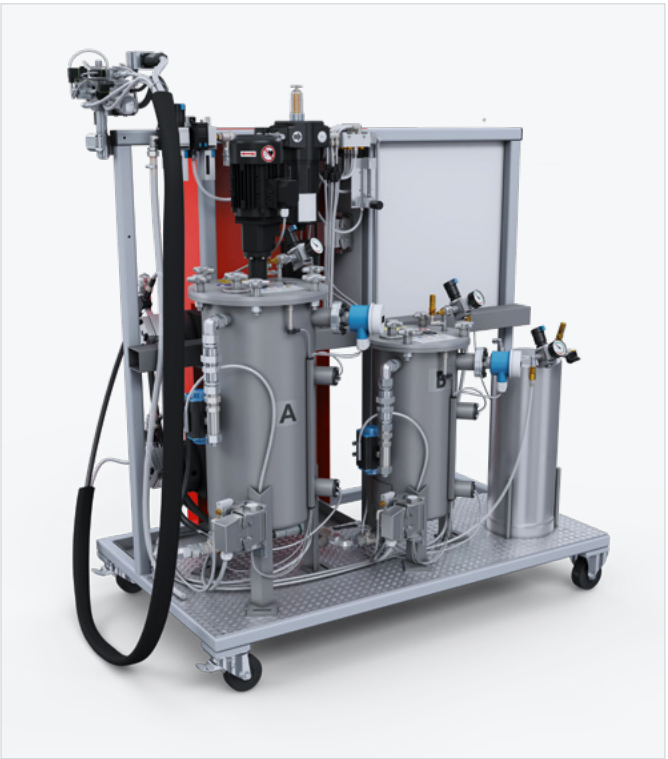
The DM 70 COMPACT mixing and dosing machine with material pressure tanks (24 l or 44 l), equipped with minimum fill level sensors and an additional pressure tank for the mixing head cleaning agent
