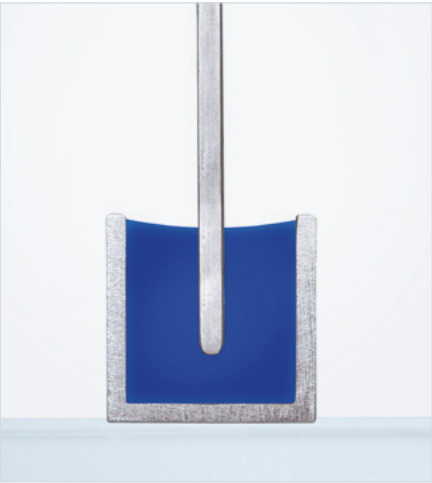
Cross-section: Tongue immersed in polyurethane gel seal
