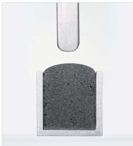
Cross-section of a polyurethane foam bead in the groove without pressing
