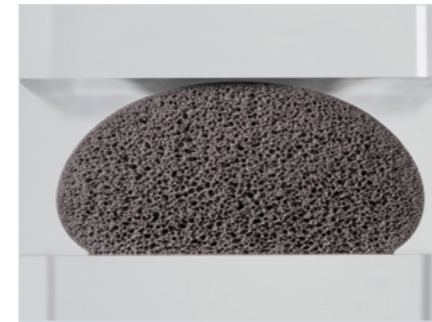
Cross-section of a polyurethane foam bead – unpressed
