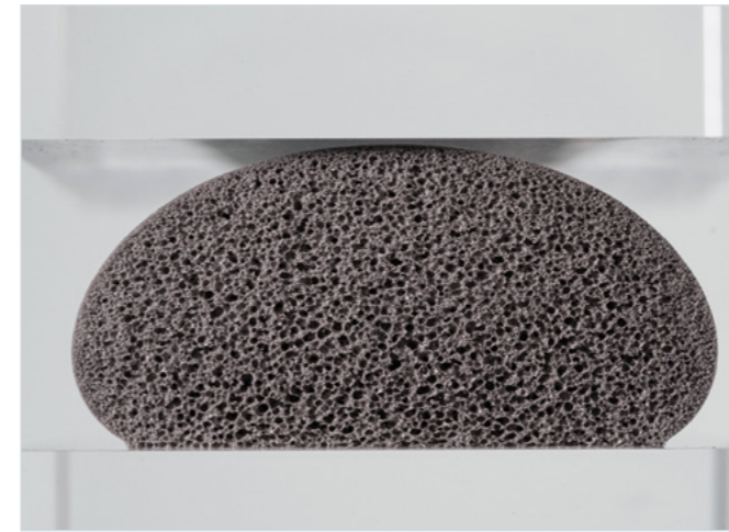
Cross-section of a polyurethane foam bead – unpressed
