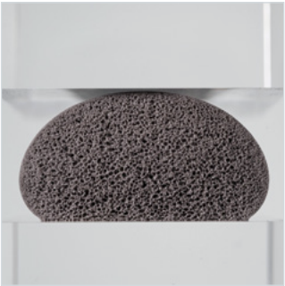
Cross-section of a polyurethane foam bead – uncompressed
