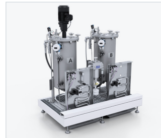
Separate standing material pressure tanks (24 L or 44 L, single-walled or double-walled) with capacitive minimum fill level sensors, on grating platform, with adjustable leveling feet and drip pan
